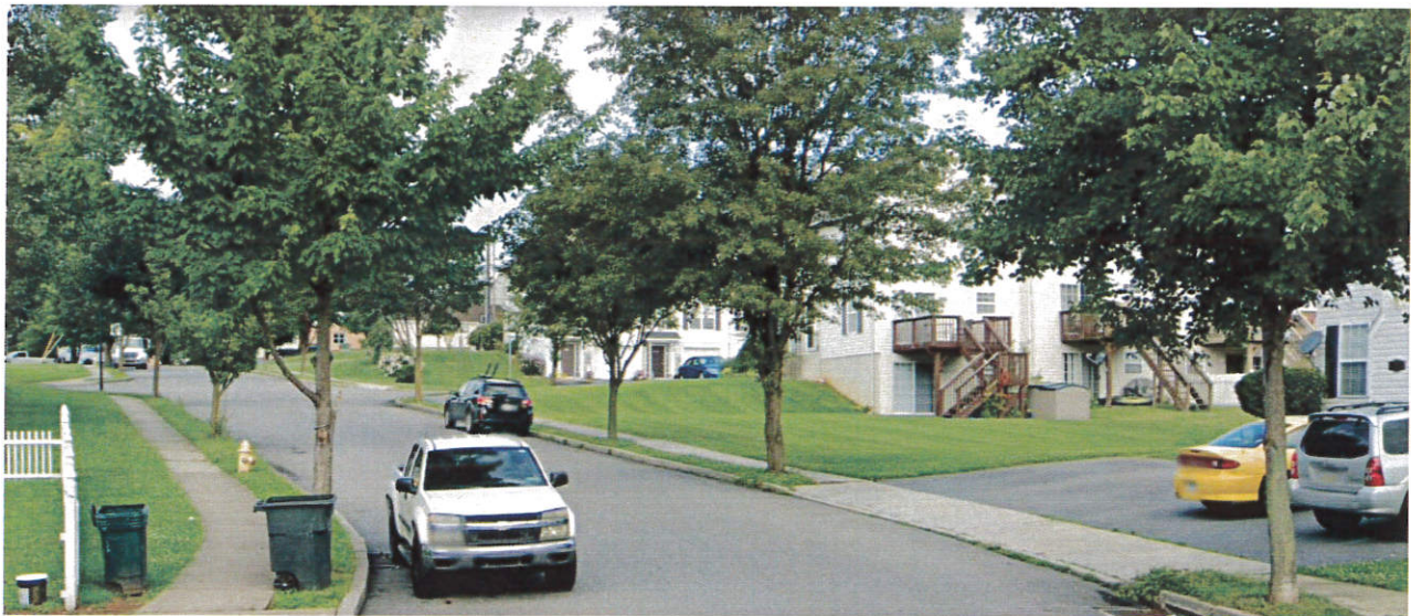
Picture 1. Typical existing parking conditions along Ramblewood Lane, reducing roadway width and sight distance on the horizontal curve.
